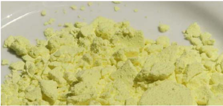
Figure 8: Produced Sulphur from the Surface Pilot Unit.
